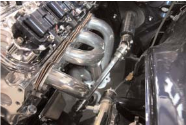
S&P makes these Chromex coated headers to clear the steering rod for rack & pinions set up among many other special applications.
