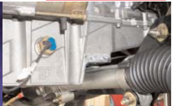
96-up 4L60E 6 Bolt to 4 Bolt Tail Housing Adapter for Manual Speedometer. Kit includes elec VSS and proper Gear Drive Gear ratio and tire rollout is needed when ordering.
